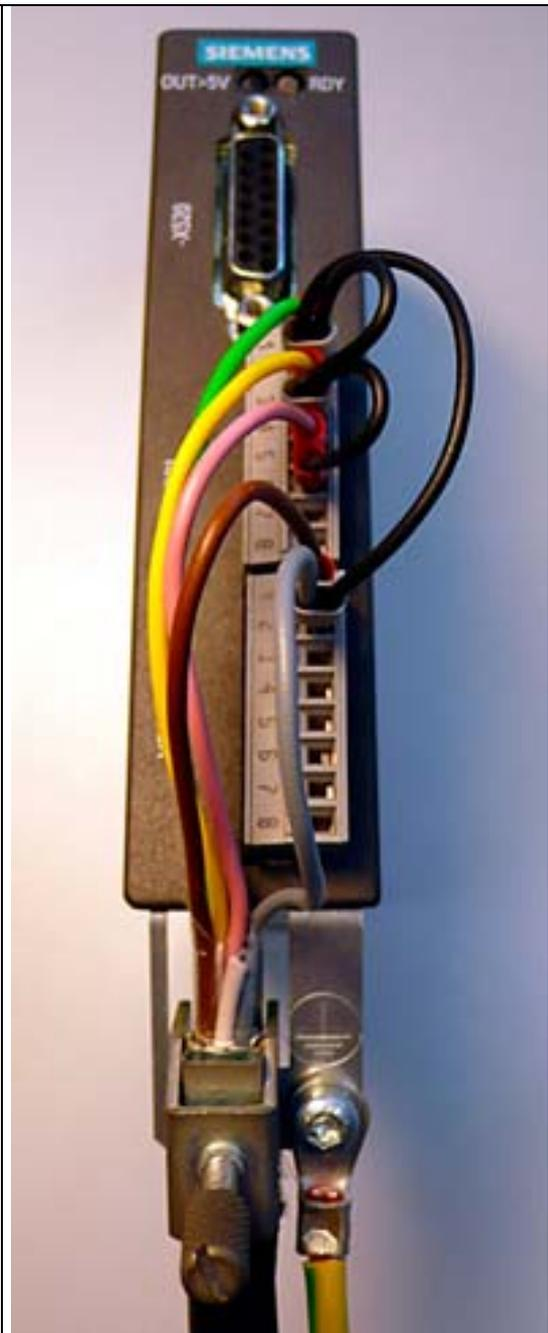
Photo of connection example 2: SMC30, 50 mm wide (Order No. 6SL3055-0AA00-5CA0, 6SL3055-0AA00-5CA1)
