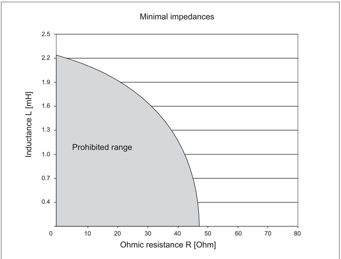
Figure 4-10 Connectable impedances with an excitation frequency  $f = 5000$  Hz
