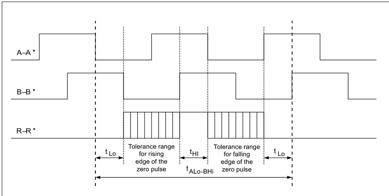
Figure 4-27 Position of the zero pulse to the track signals
