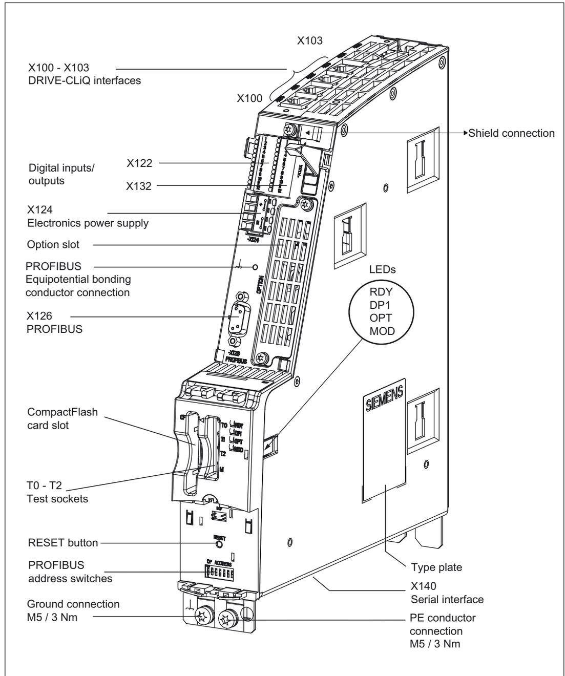
Figure 2-3 Interface description of the CU320 (covers removed)
