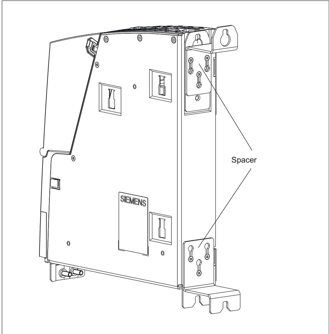
Figure 2-10 Installing the CU320 on a mounting surface using spacer elements
