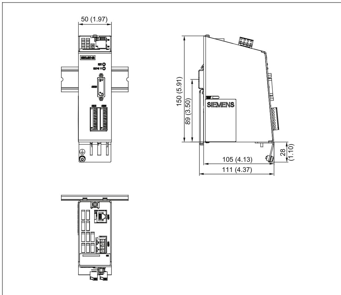
Figure 4-21 Dimension drawing SMC30: 50 mm wide
