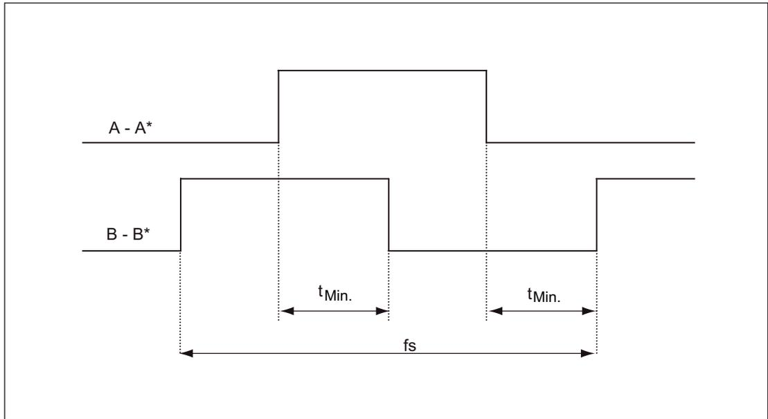
Figure 4-26 Signal characteristic of track A and track B between two edges: Time between two edges with pulse encoders
