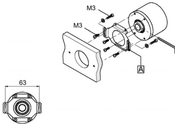
Figure 4-55 Installation: Hollow shaft, A: Spring plate (included in scope of supply)
