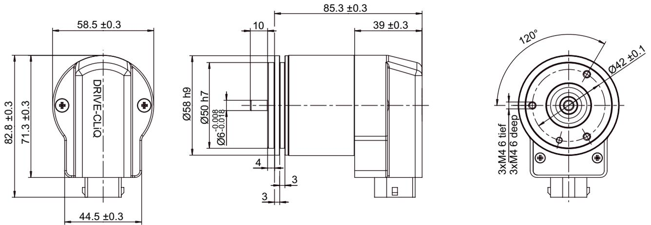
Figure 4-51 Dimension drawing: Synchronous flange
