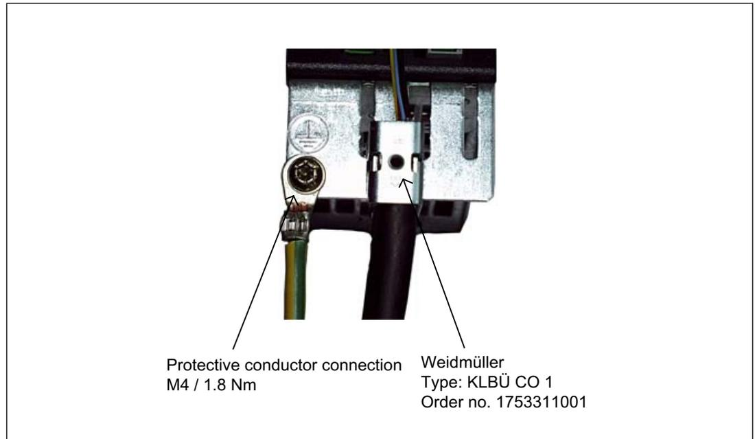
Figure 4-24 Shield contacts for the SMC30
