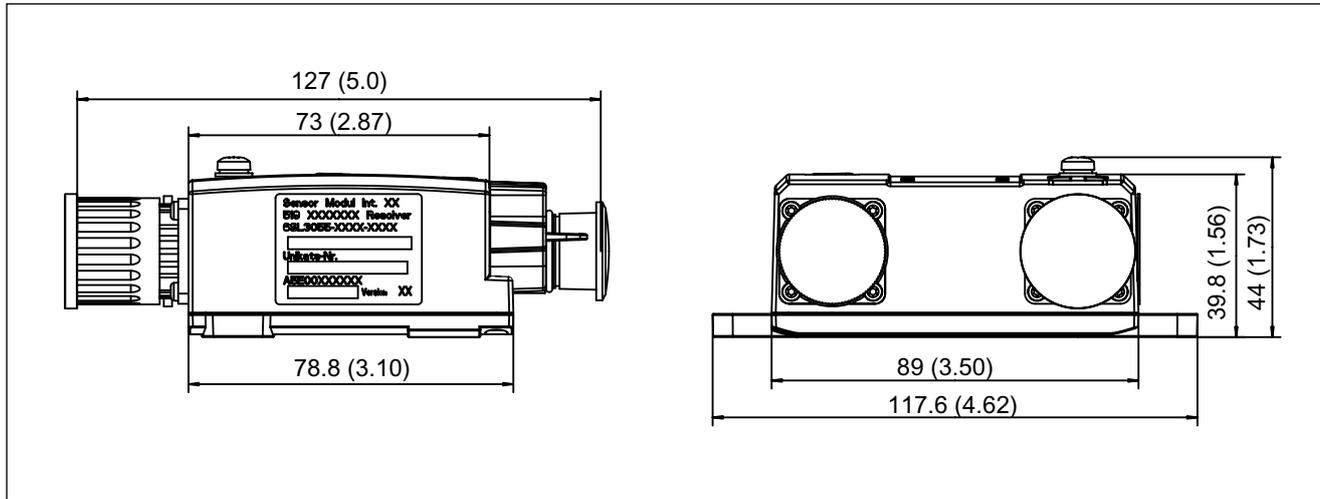
Figure 4-47 Dimension drawing SME125, Order number 6SL3055-0AA00-5KA0
