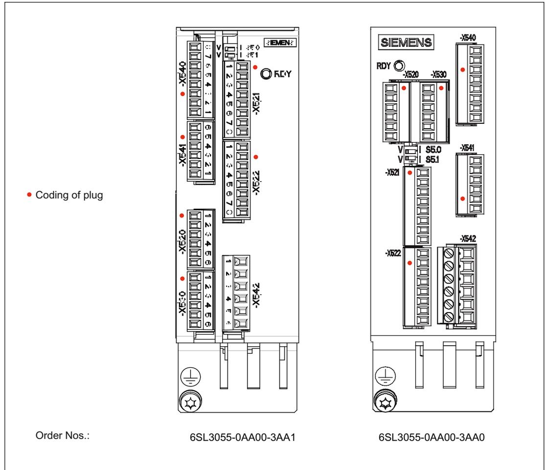
Figure 3-25 Connector codes of the TM31
