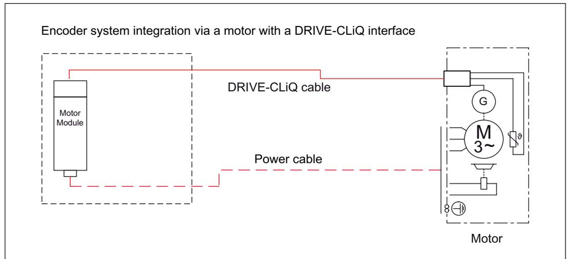
Figure 4-4 Encoder system integration via a motor with a DRIVE-CLiQ interface
