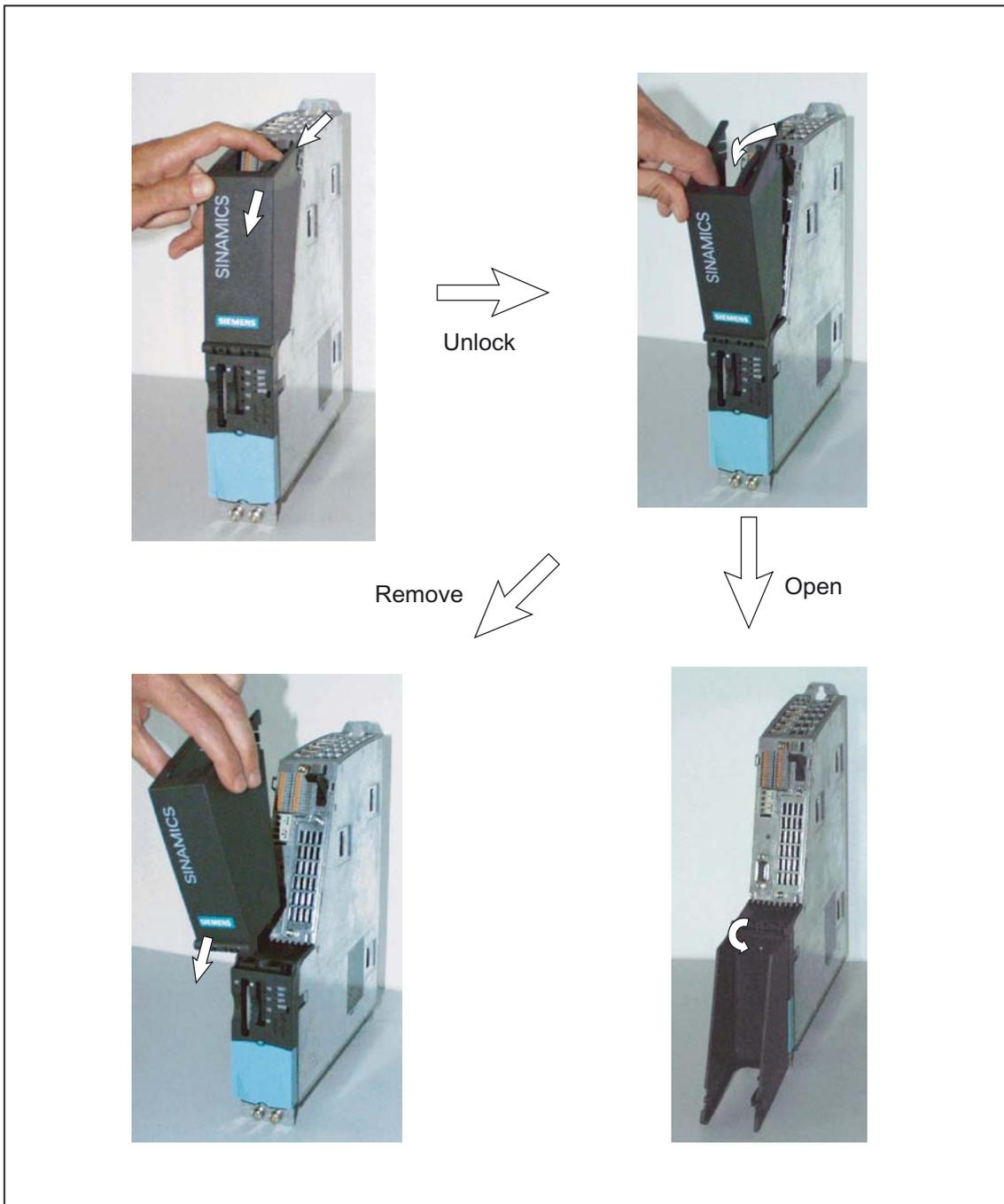
Figure 2-11 Removing/opening the cover of the CU320
