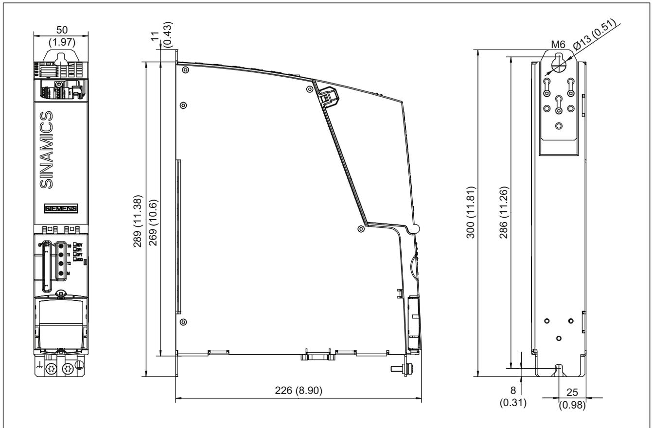
Figure 2-7 Dimension drawing: CU320
