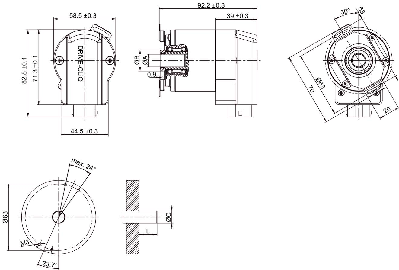
Figure 4-53 Dimension drawing: Hollow shaft with blind bore
