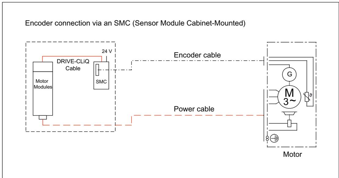
Figure 4-3 Encoder connection via an SMC (Sensor Module Cabinet-Mounted)
