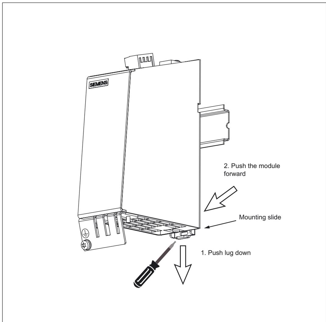
Figure 3-46 Releasing the component from a DIN rail
