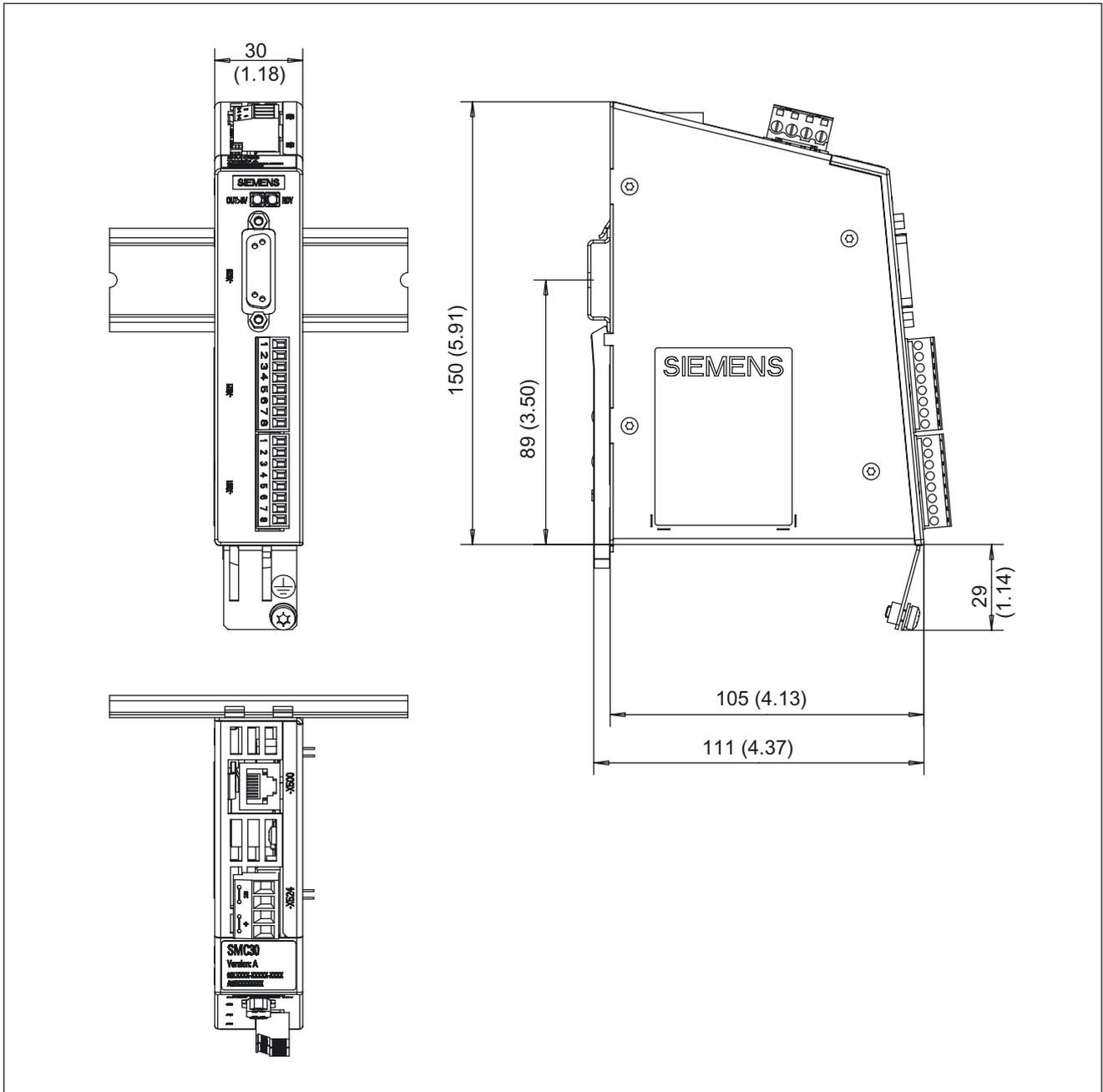
Figure 4-20 Dimension drawing SMC30: 30 mm wide
