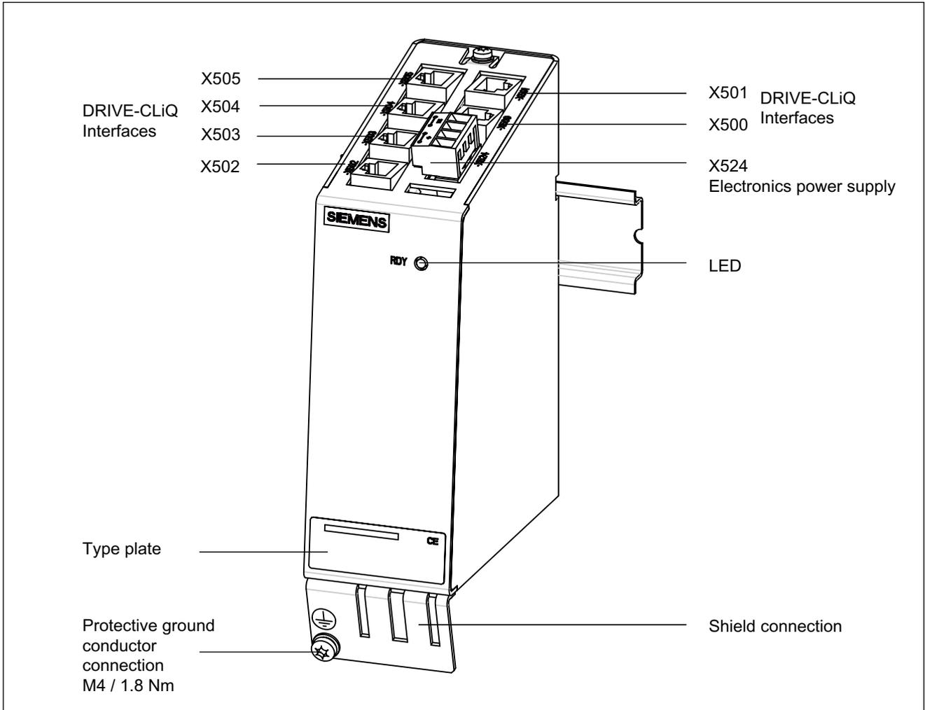
Figure 3-37 Interface description of the DMC20
