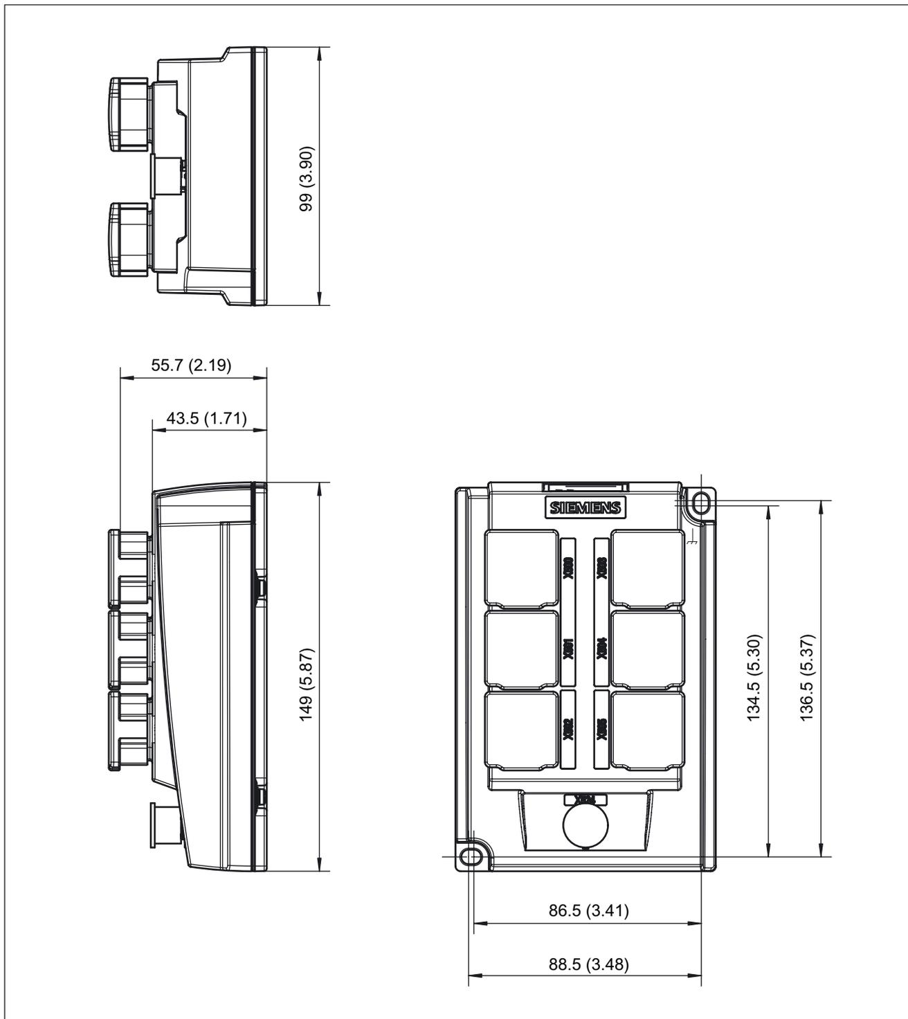
Figure 3-41 Dimension drawing: DME20
