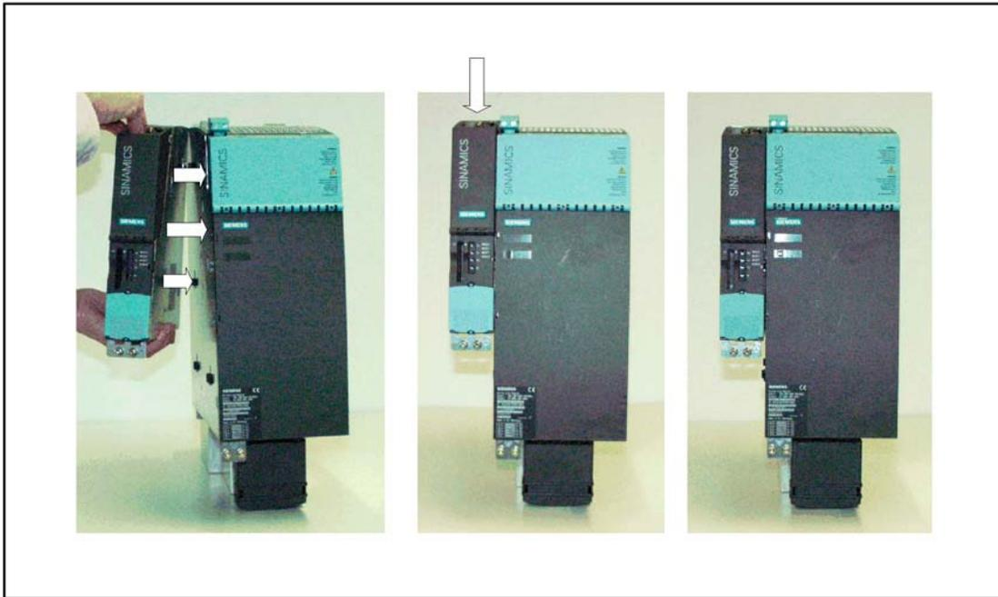
Figure 2-8 Mounting the CU320 directly on a Line Module in booksize format
