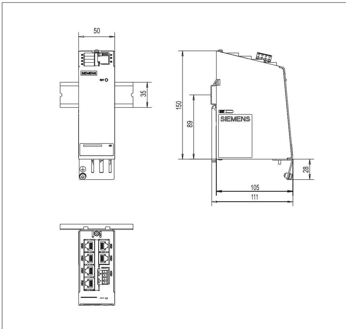
Figure 3-38 Dimension drawing of the DMC20
