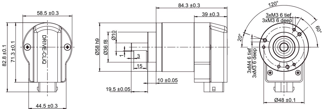
Figure 4-52 Dimension drawing: Clamping flange
