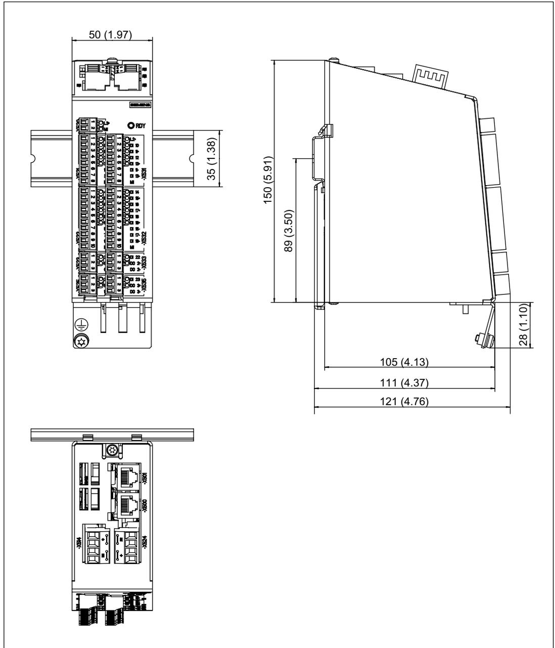
Figure 3-35 Dimension drawing of TM54F
