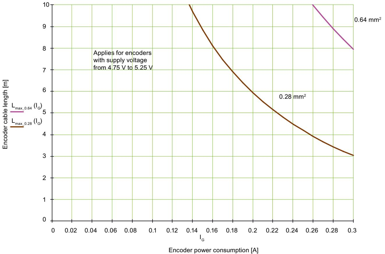
Figure 4-32 Max. cable length as a function of the current drawn by the encoder system
