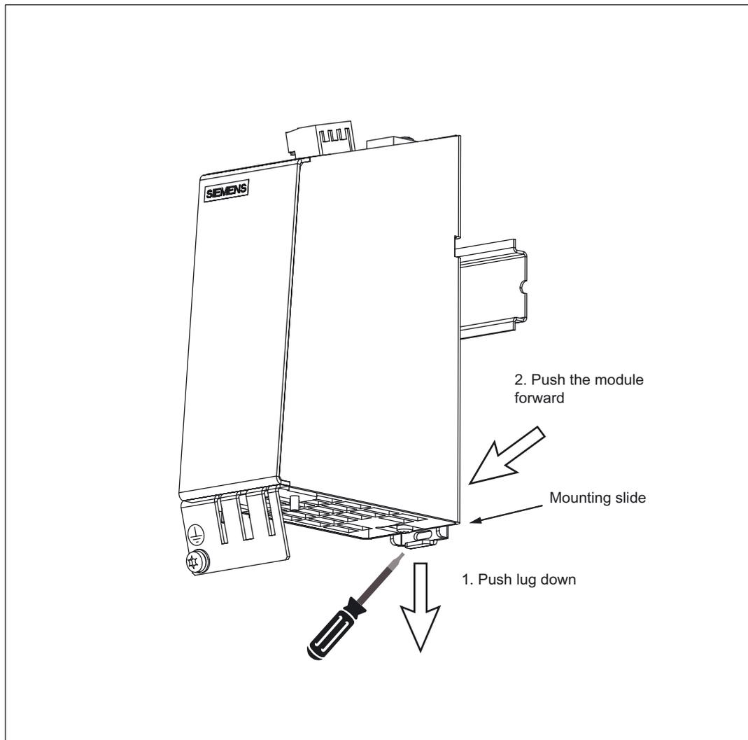
Figure 3-36 Releasing the component from a DIN rail
