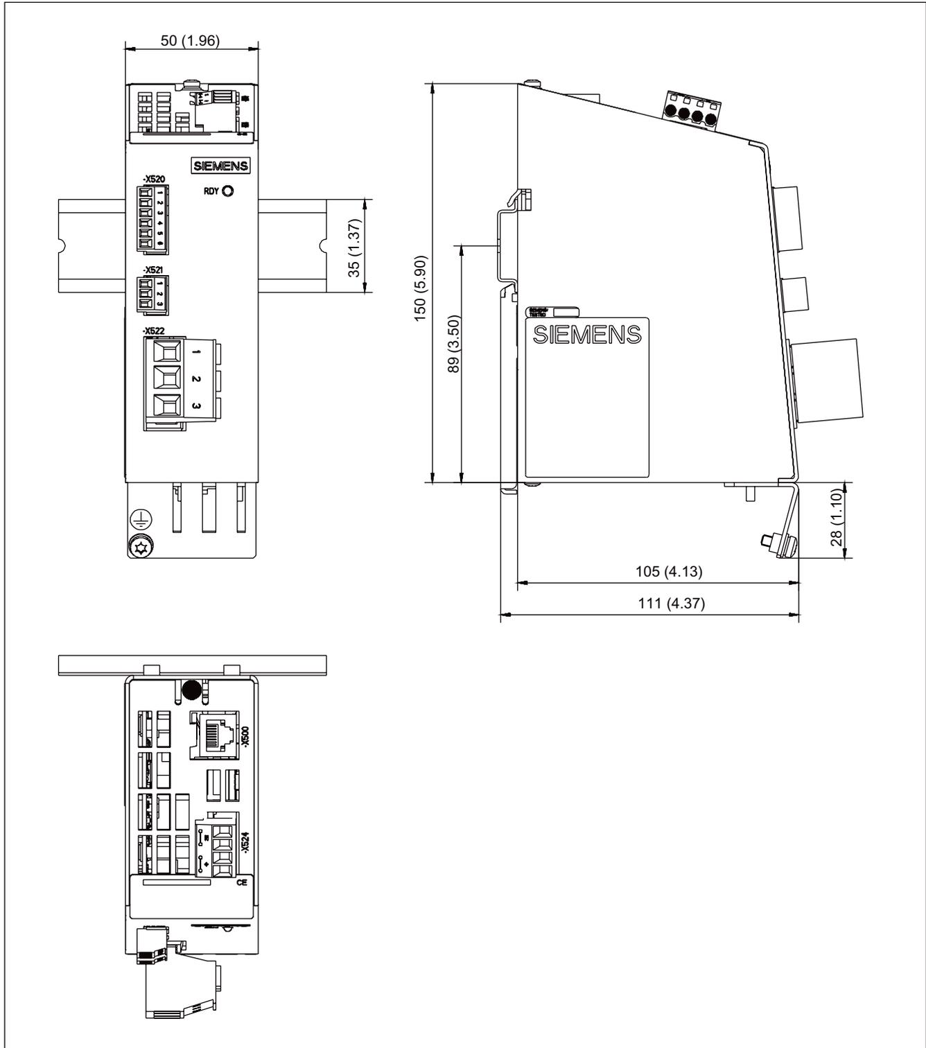
Figure 3-45 Dimension drawing: Voltage Sensing Module
