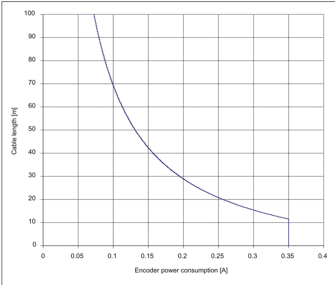
Figure 4-25 Max. cable length as a function of the encoder current drawn
