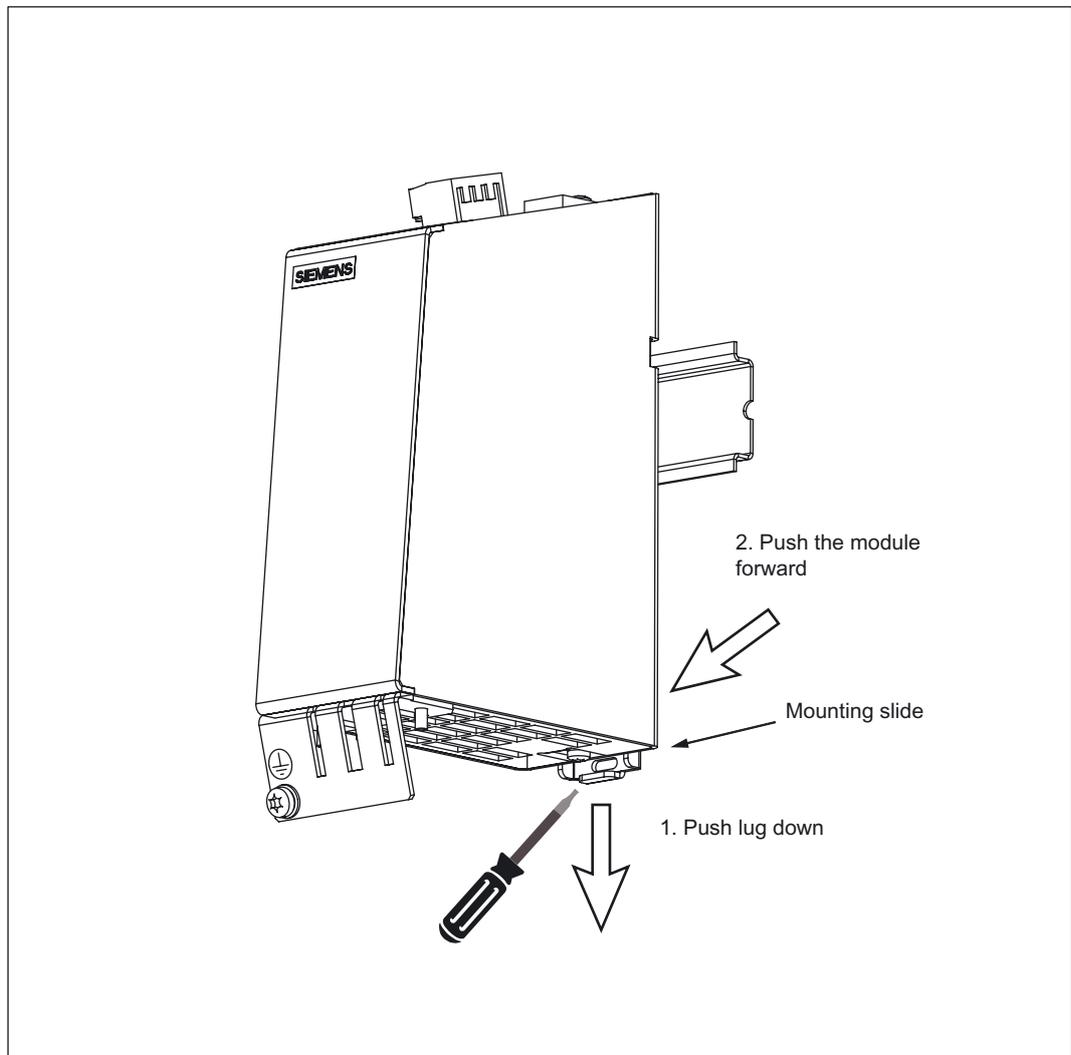
Figure 4-9 Releasing the component from a DIN rail
