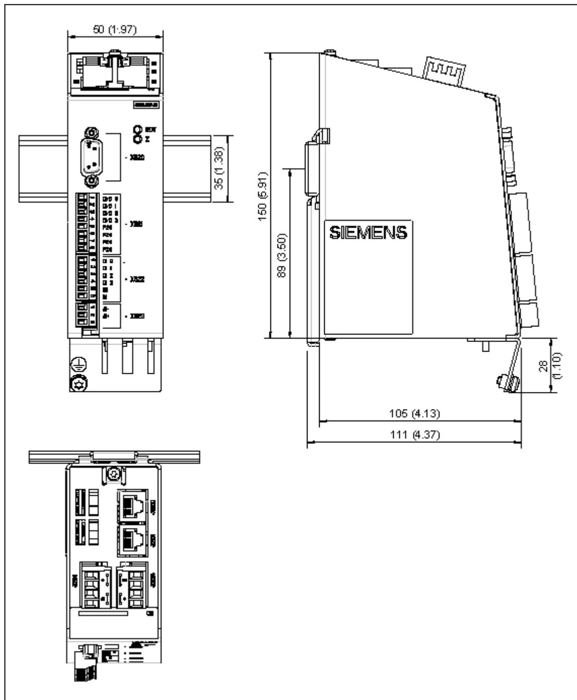
Figure 3-29 Dimension drawing TM41, Order number 6SL3055-0AA00-3PA1
