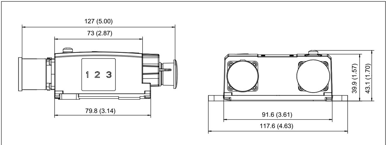
Figure 4-46 Dimension drawing SME125, Order number 6SL3055-0AA00-5KA3
