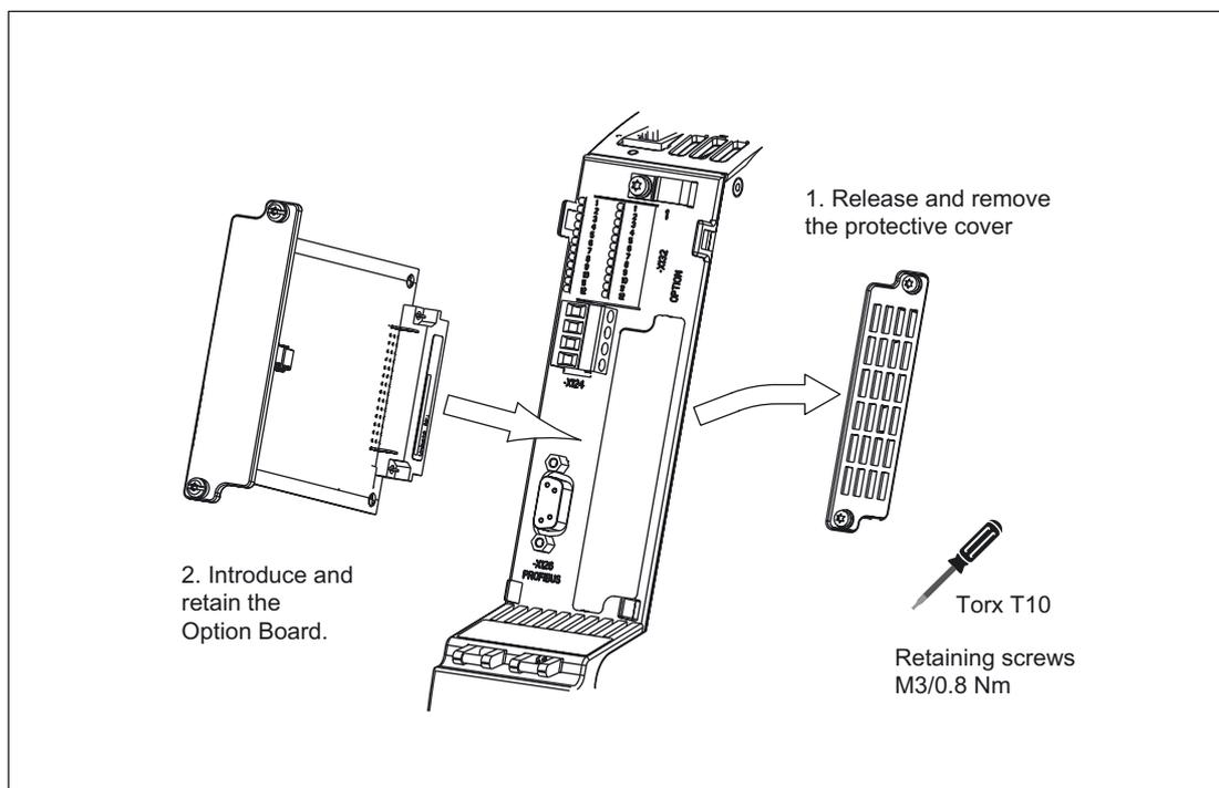
Figure 3-5 Installation of an option board in a CU320
