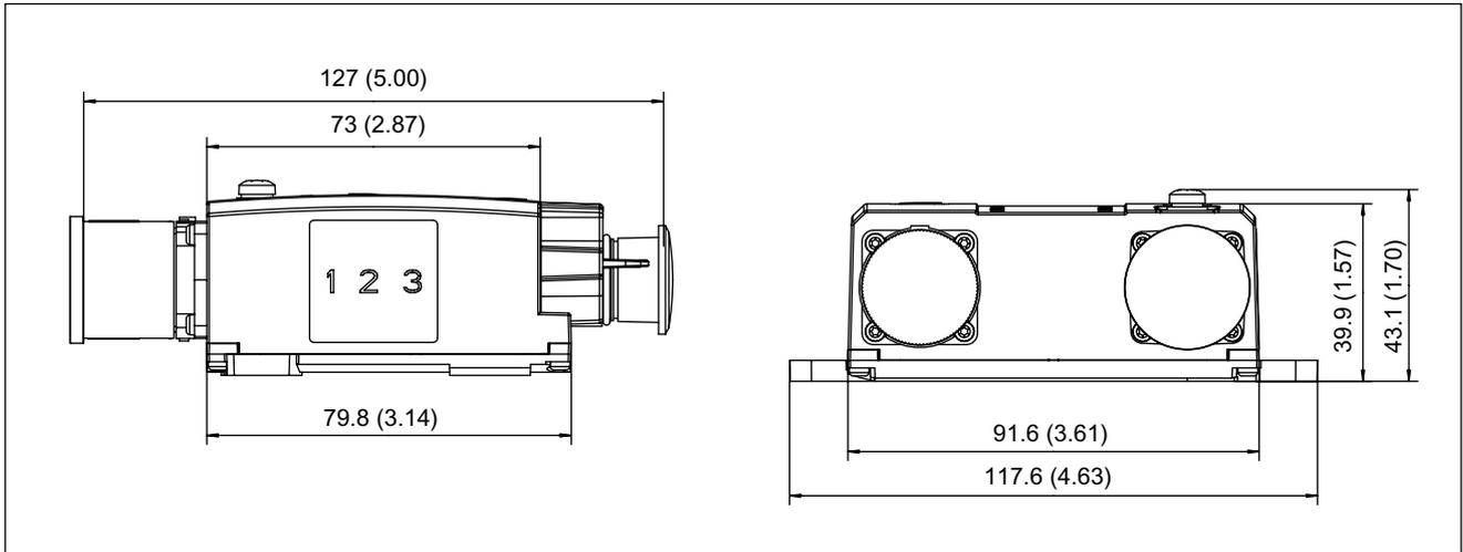
Figure 4-40 Dimension drawing SME120, Order number 6SL3055-0AA00-5JA3
