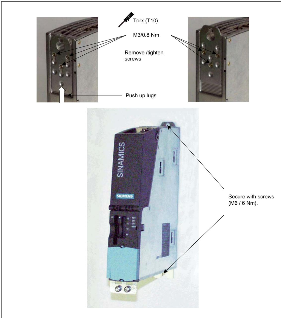
Figure 2-9 Installing the CU320 directly on a mounting surface
