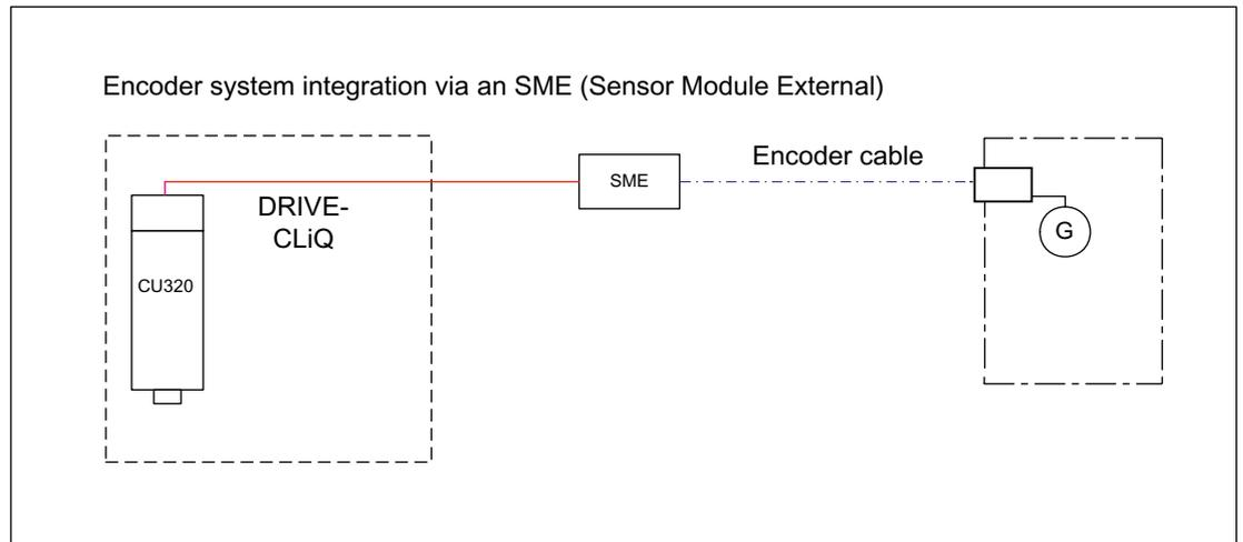
Figure 4-5 Encoder system integration via an SME (Sensor Module External)
