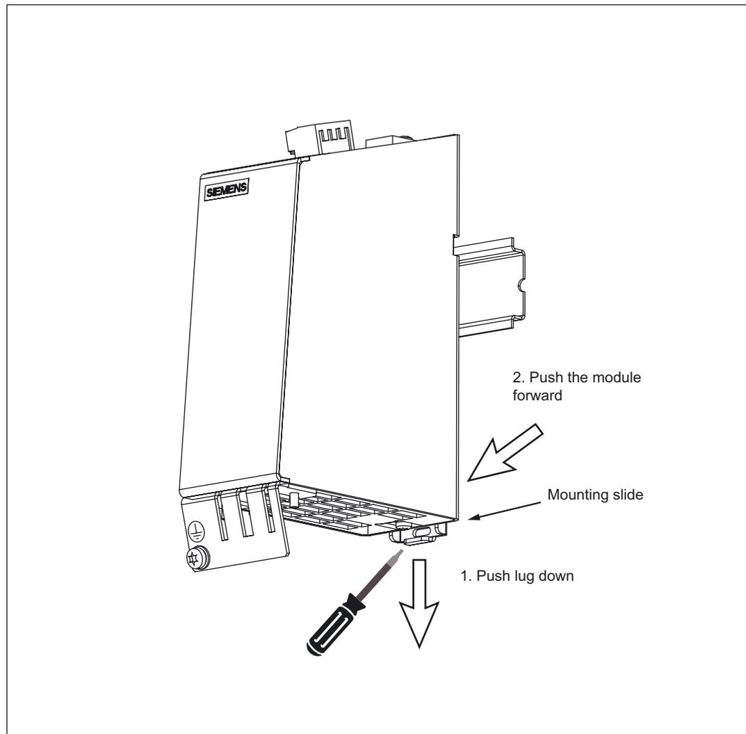
Figure 3-15 Releasing the component from a DIN rail
