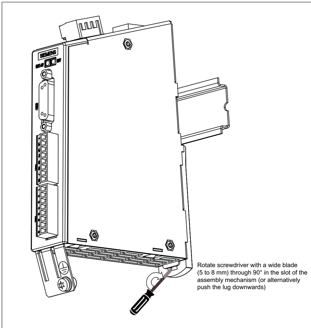
Figure 4-23 Removing: SMC30: 30 mm wide
