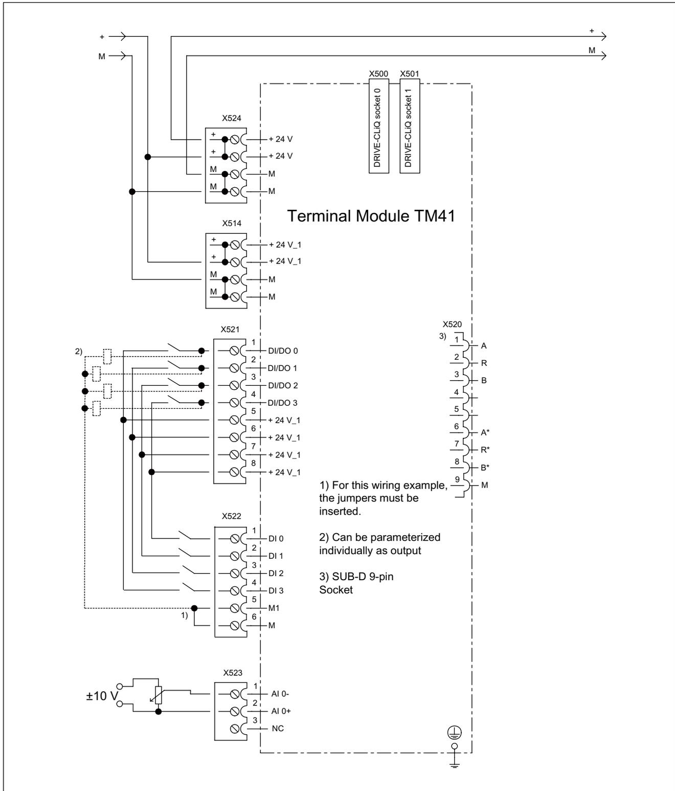
Figure 3-28 Sample connection of TM41
