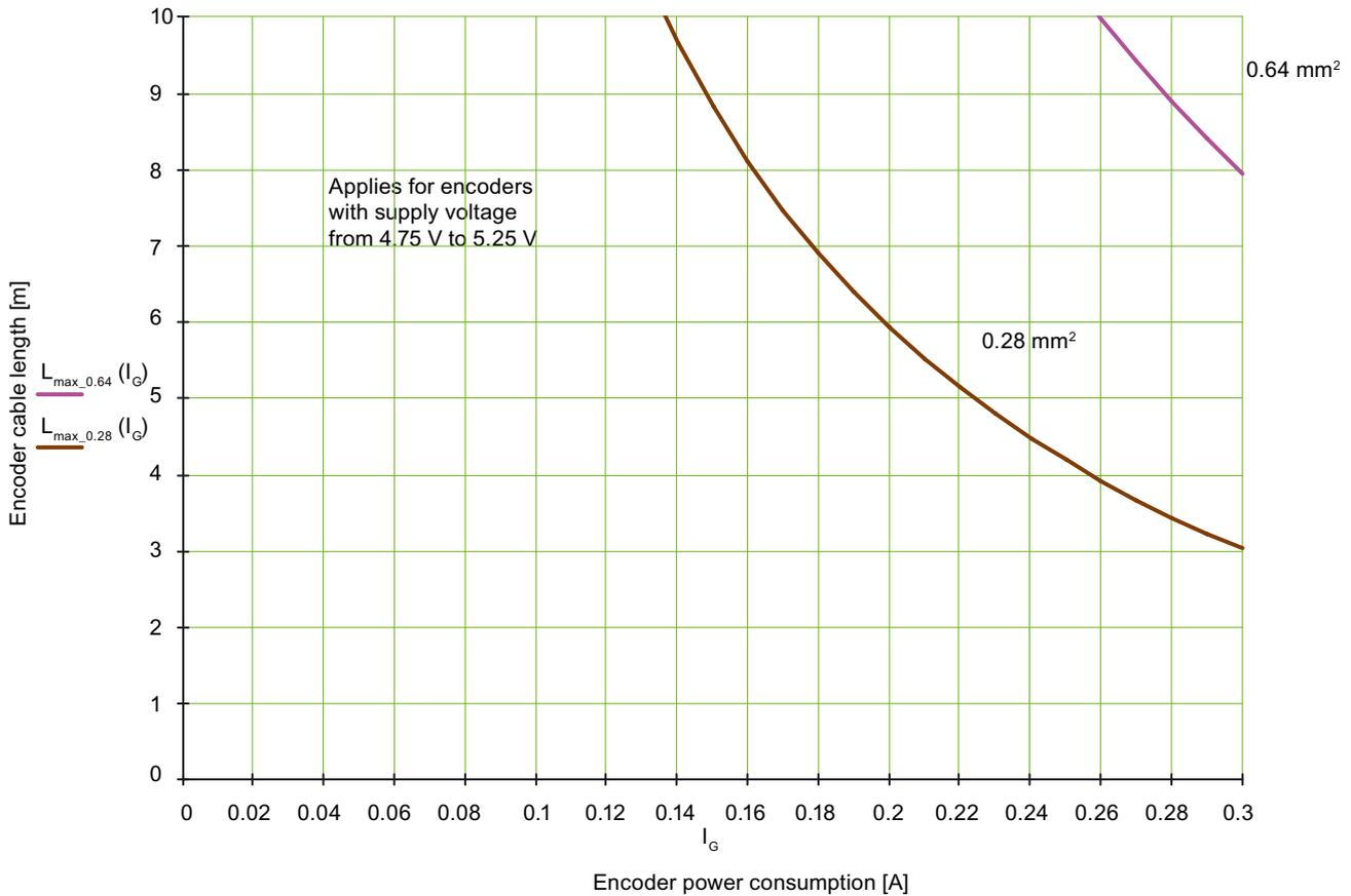
Figure 4-49 Max. cable length as a function of the current drawn by the encoder system
