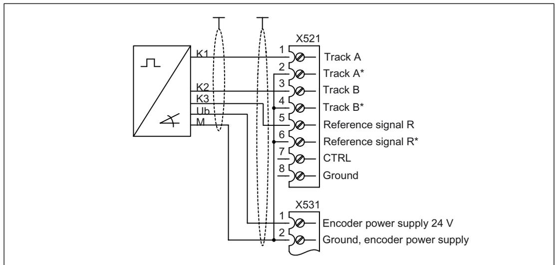
Figure 4-19 Connection example 2: HTL encoder, unipolar, with reference signal<sup>1)</sup>
