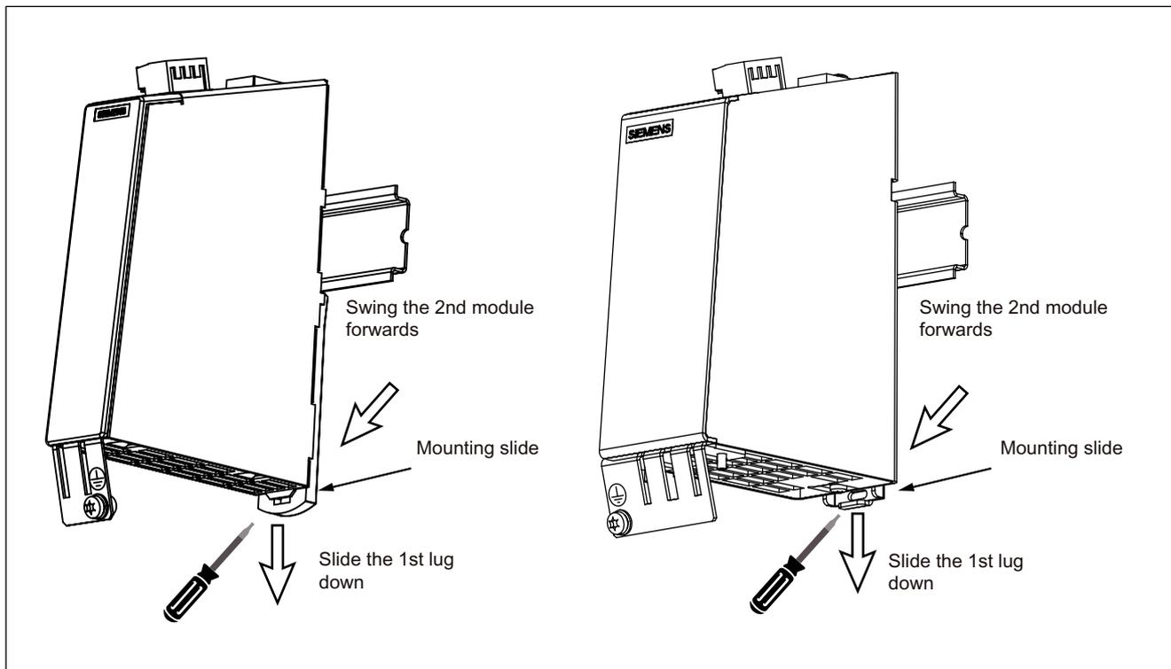
Figure 4-15 Disassembly of a DIN rail with a 30mm wide component (left) and with a 50mm wide component (right).
