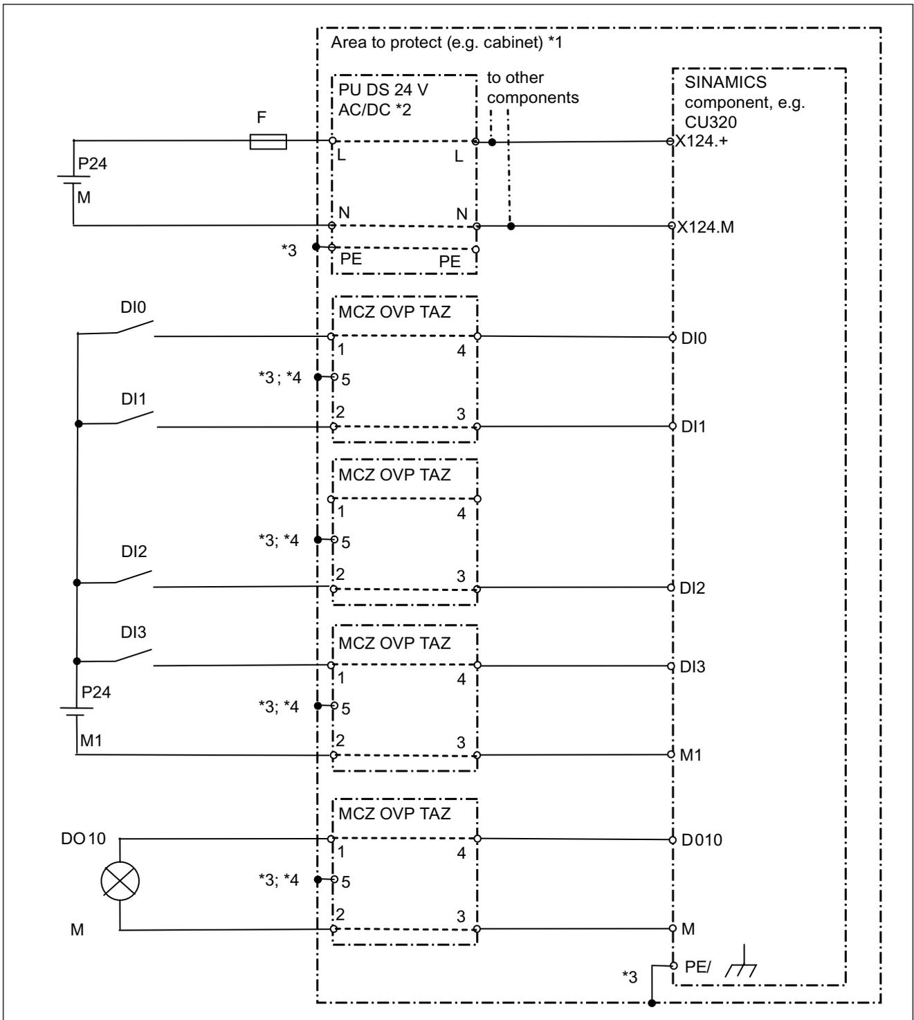
Figure 2-5 Connection example: Overvoltage protection components from Weidmüller to SINAMICS components
