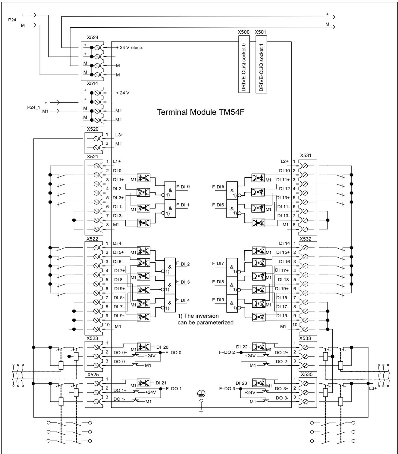
Figure 3-34 Connection example: TM54F
