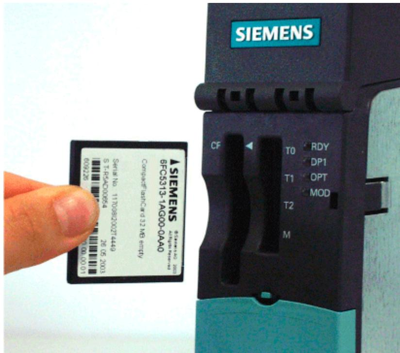
Figure 2-6 CompactFlash card slot
