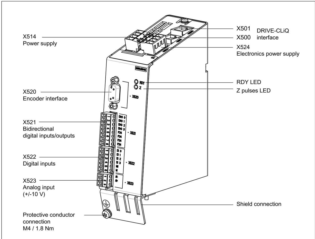
Figure 3-26 TM41 interface description, Order number 6SL3055-0AA00-3PA1
