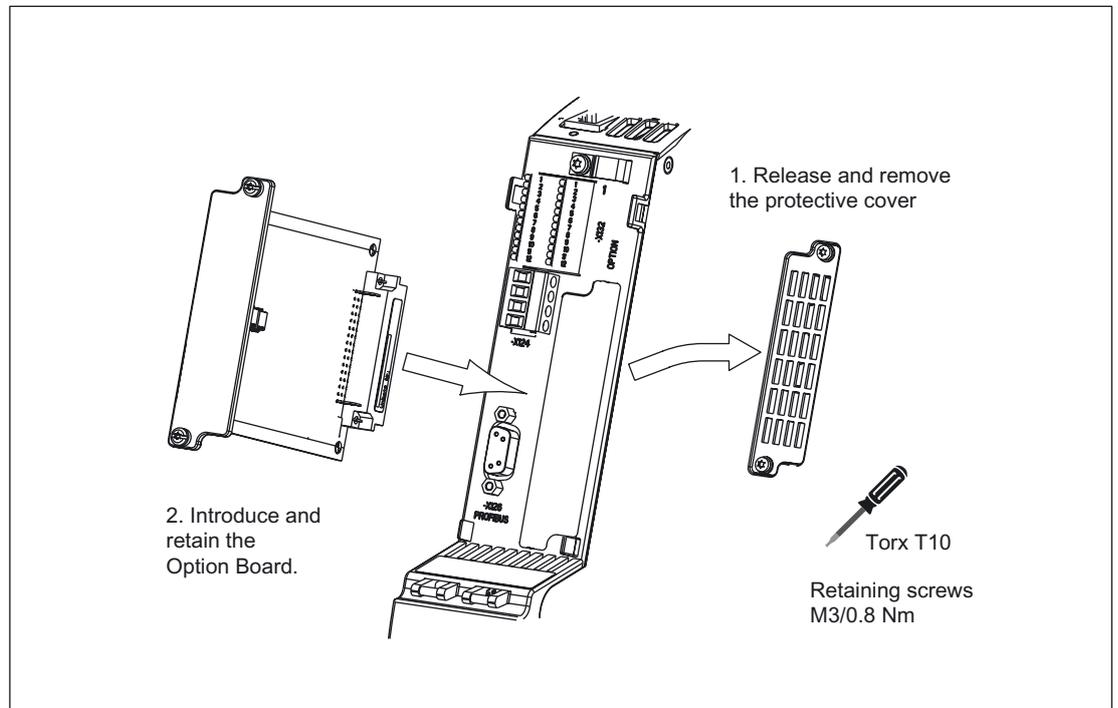
Figure 3-10 Installation of an option board in a CU320
