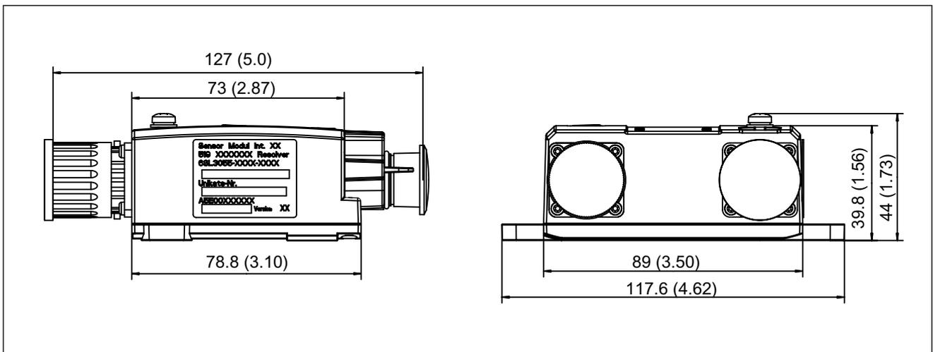
Figure 4-41 Dimension drawing SME120, Order number 6SL3055-0AA00-5JA0
