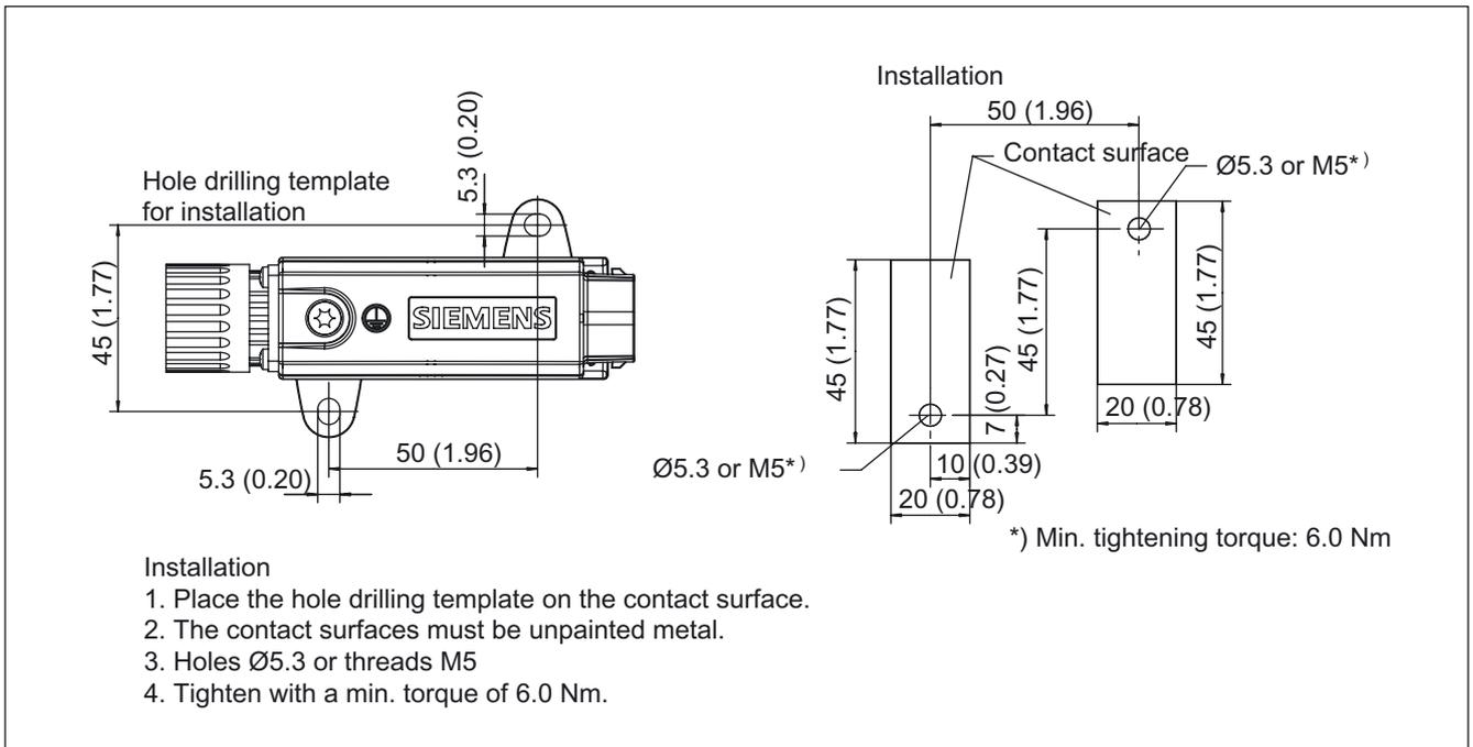
Figure 4-36 Installing the SME20/SME25
