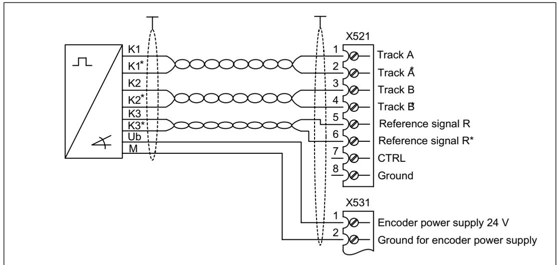
Figure 4-18 Connection example 1: HTL encoder, bipolar, with reference signal
