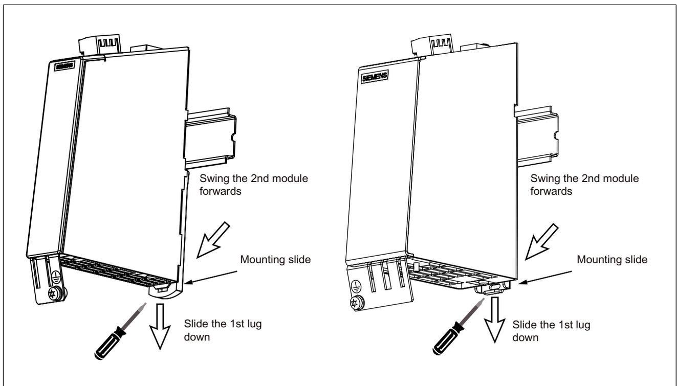
Figure 4-22 Disassembly of a DIN rail with a 30mm wide component (left) and with a 50mm wide component (right).
