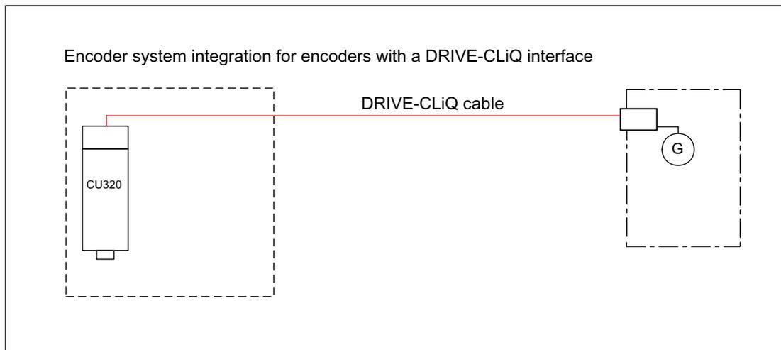
Figure 4-6 Encoder system integration of encoders with DRIVE-CLiQ interface (e.g. DRIVE-CLiQ encoder)
