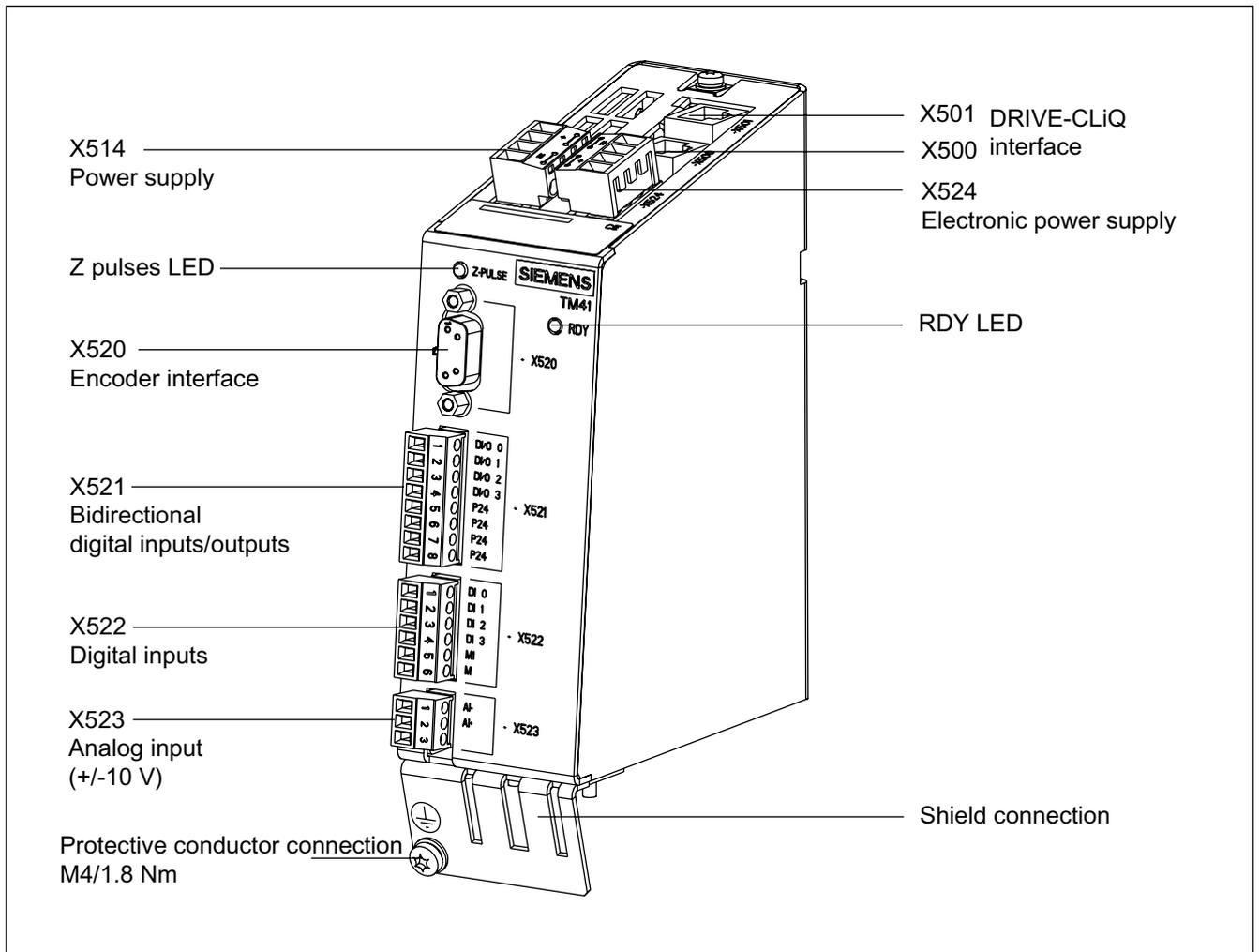
Figure 3-27 TM41 interface description, Order number 6SL3055-0AA00-3PA0
