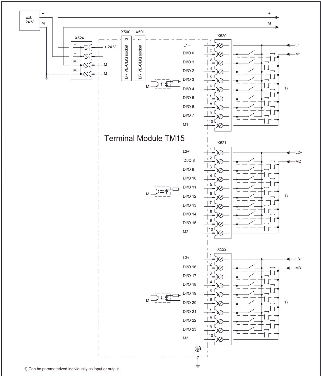
Figure 3-13 Example connection of TM15
