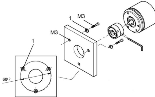
Figure 4-54 Installation: Synchronous flange, 1: Clamp straps
