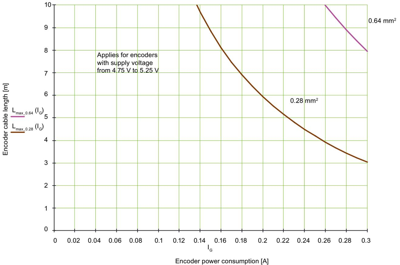
Figure 4-37 Max. cable length as a function of the current drawn by the encoder system
