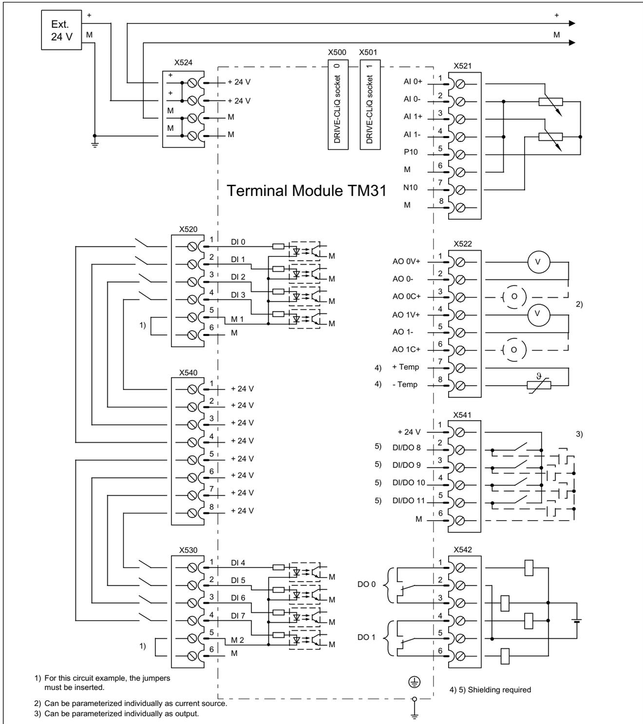
Figure 3-20 Example connection of TM31
