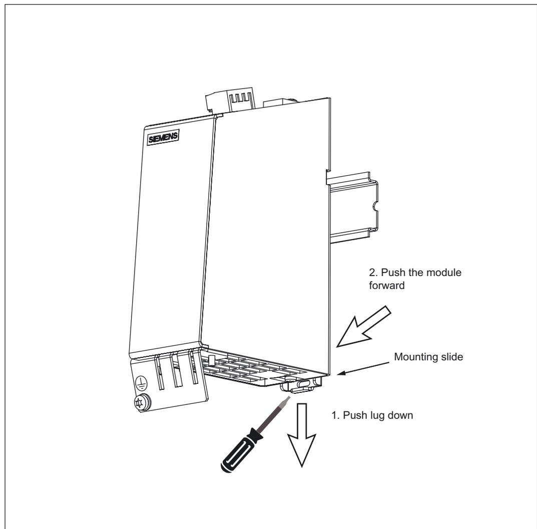
Figure 3-23 Releasing the component from a DIN rail
