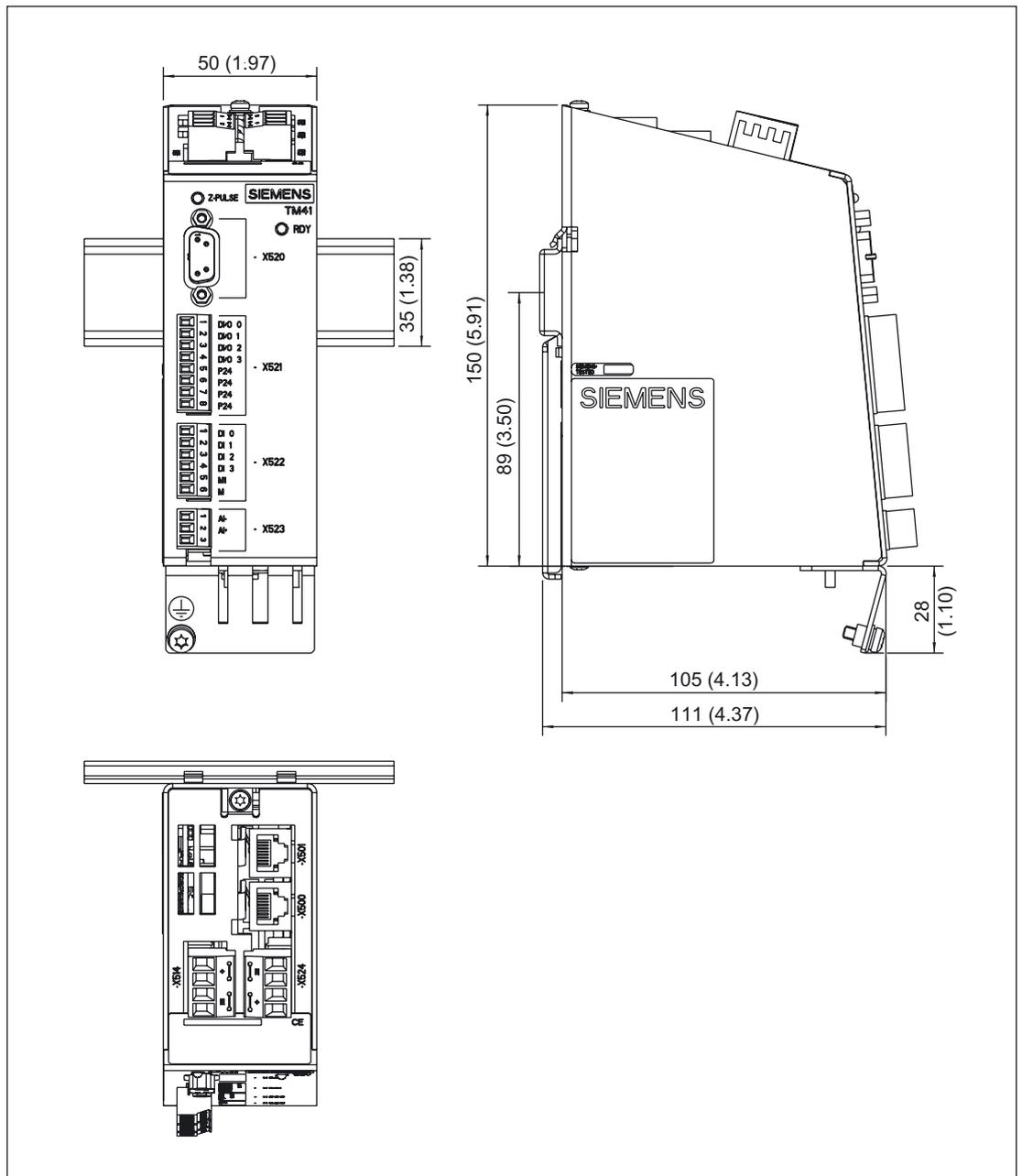
Figure 3-30 Dimension drawing TM41, Order number 6SL3055-0AA00-3PA0
